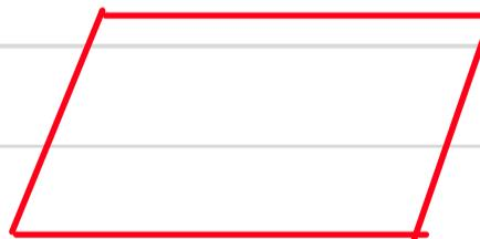
Used to perform input or output
