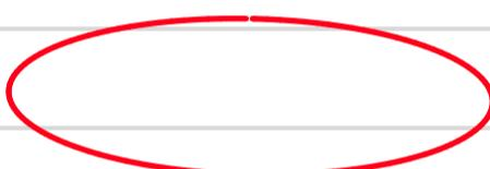
Used for start or stop of an algorithm
